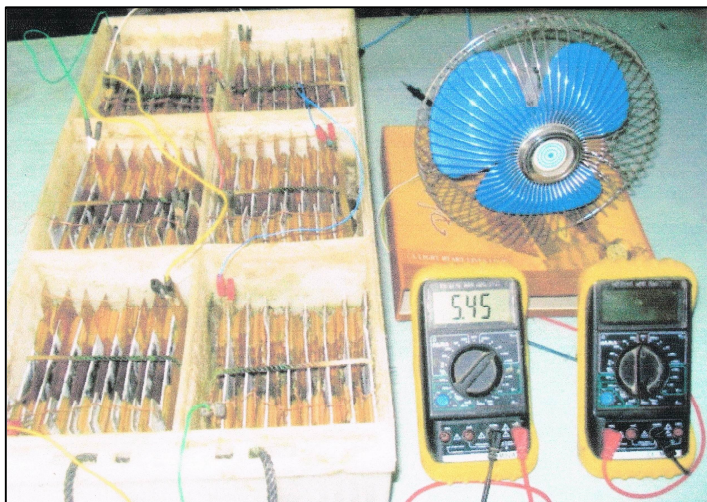
Figure: Preperation of BPL/PKL Electricity Module
